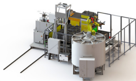
Gleason Automations Systems provides protective guarding around the loading area to provide a safe work environment.
